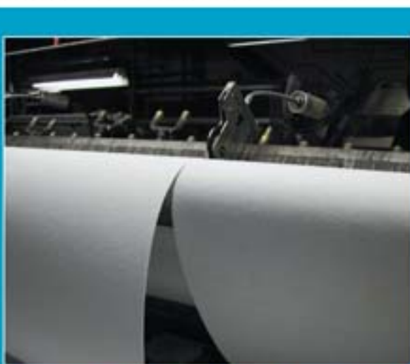
A nonwoven roll being split on one of PCC's machines. The company supplies a variety of products for the home furnishing market.
